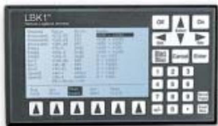
The optional LBK1 Remote Operation Terminal provides control of the LogBook system in the field when no PC is present
