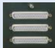
DB37-style termination panel (DBK608) features three standard 37-pin female connectors
