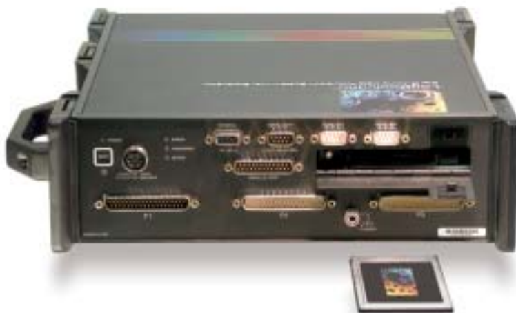
One PC-Card can be removed and another PC-Card inserted without causing a gap in the acquired data
